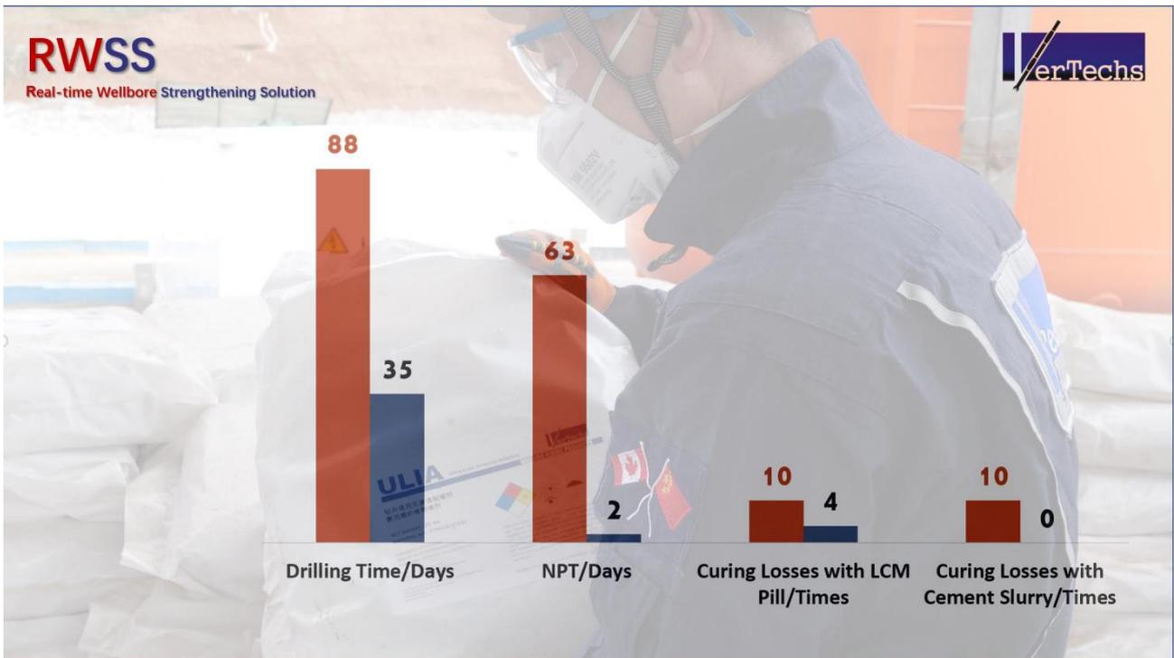
Case Study - An interval drilled with downhole complexity (Red) vs. sidetrack with Vertechs® RWSS (Blue)
